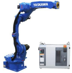
Manipulator and control box
